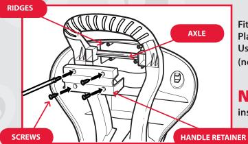
Fit axle on rear handle into ridges in underside of body. Place handle retainer over axle (retainer fits only one way). Using the 4 plain #6 screws and Phillips/cross head screwdriver (not included), attach retainer to body.
